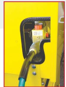
Side cable opening means drawers are not blocked by the air hose
