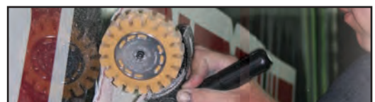
DF-702C Coarse Brush The flex allows the brushes to compress in tight corners and contour themselves over lipped edges and curved corners. Makes fast work of bed liner.
